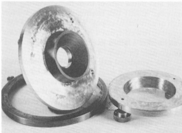
Figure 3. Rotating stage components oriented to reveal the mating annular flats and conical sections.
